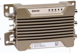
The Westermo RT-610-HV is a concurrent dual-band 802.11ac Wave2 Wireless LAN Access Point for on-board and stationary applications. It ensures reliable, high-speed data, airtime fairness, band steering, and client steering, and it can be used as a passenger hotspot or as an access point for connecting wireless industrial clients.
